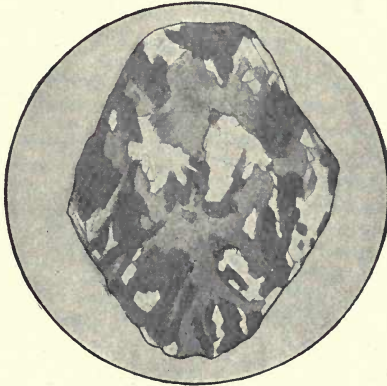
Hornblende Crystal with Partial Chloritization and Silicification; in Propylitic Andesite. Virginia City, Nevada. (After G. F. Becker.) White, quartz and calcite; grey, chlorite; dark grey, hornblende. Magnified 70 diameters.
